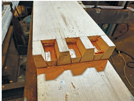
Dovetail joint in the process of being refined
