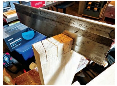
Dovetail joint sawn into the wood frame
